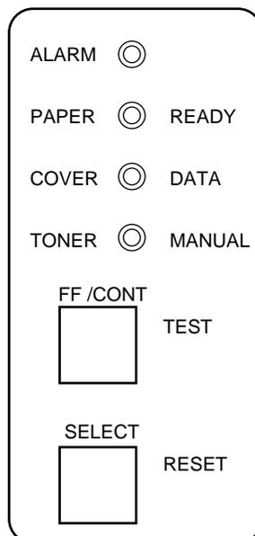
On entering this inspection mode, the LEDs show the statuses of the respective sensors.
