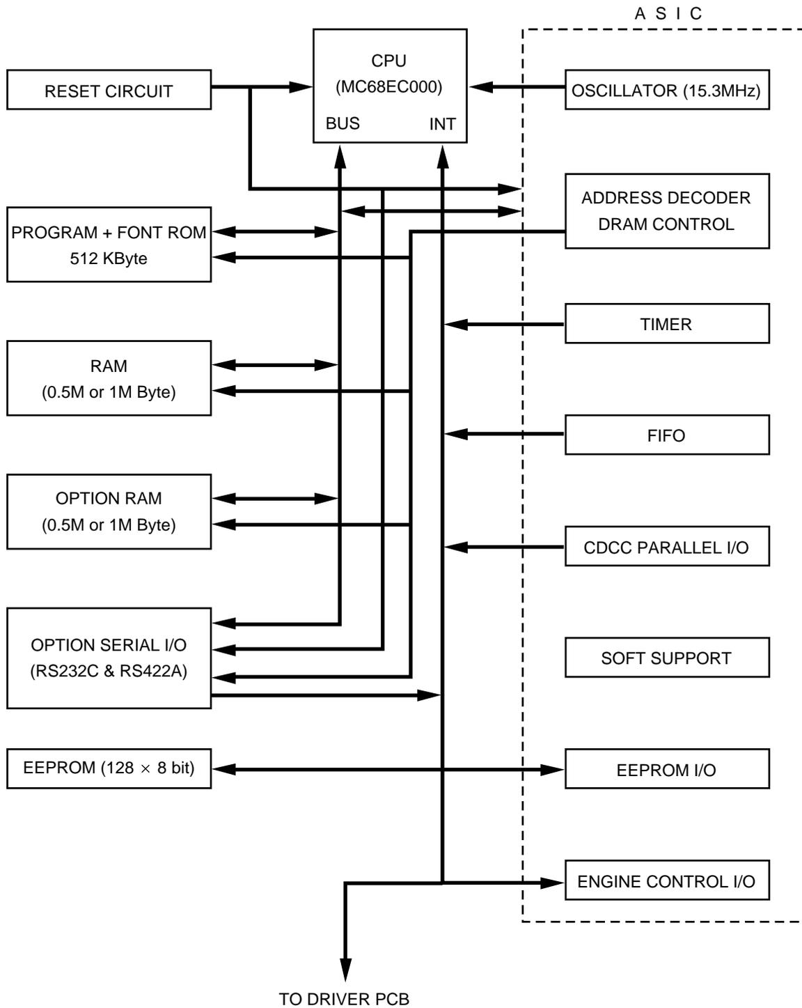
Fig. 2.2 Main PCB Block Diagram
