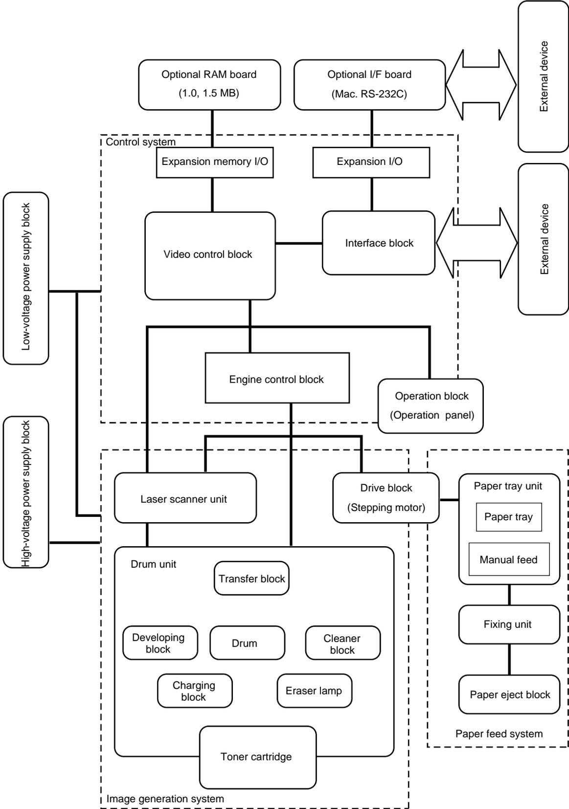
Fig. 2.1 General Block Diagram
